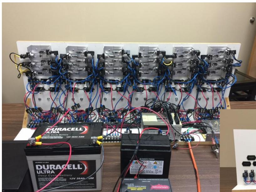
The test station as seen from the back which includes the bulbs and PLC and from the front with the relays and counters.
